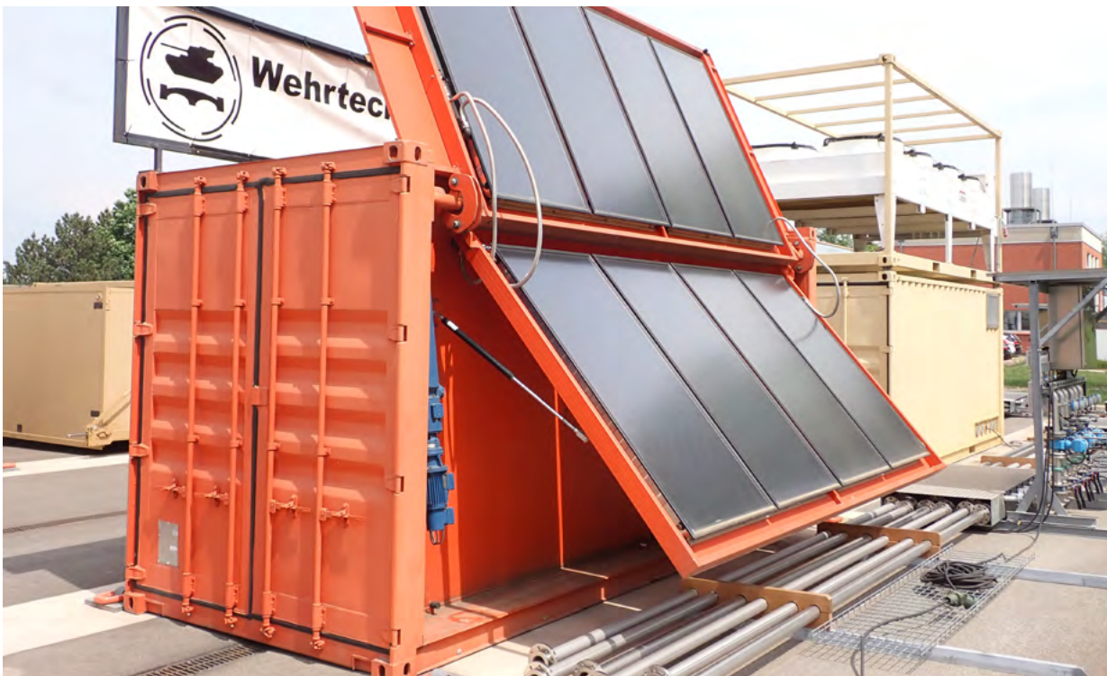
Figure 27: Solar thermal containers from the energy camp for test purposes; Source: Bundeswehr
